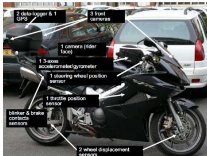
Figure 88: PTW instruments and data logger used for Naturalistic Driving 83
