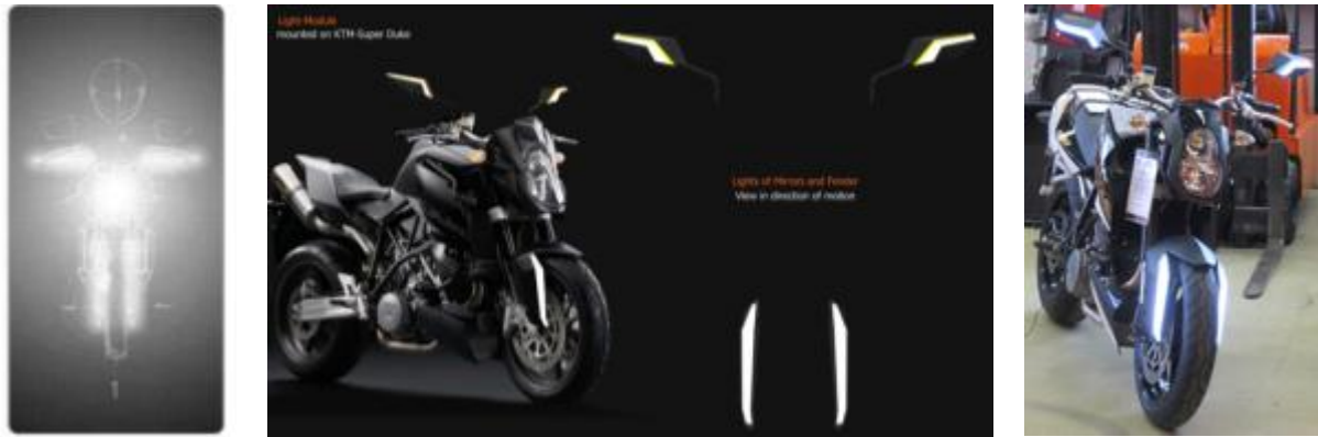
Figure 57: Alternative Front Light Patterns; T-light configuration
