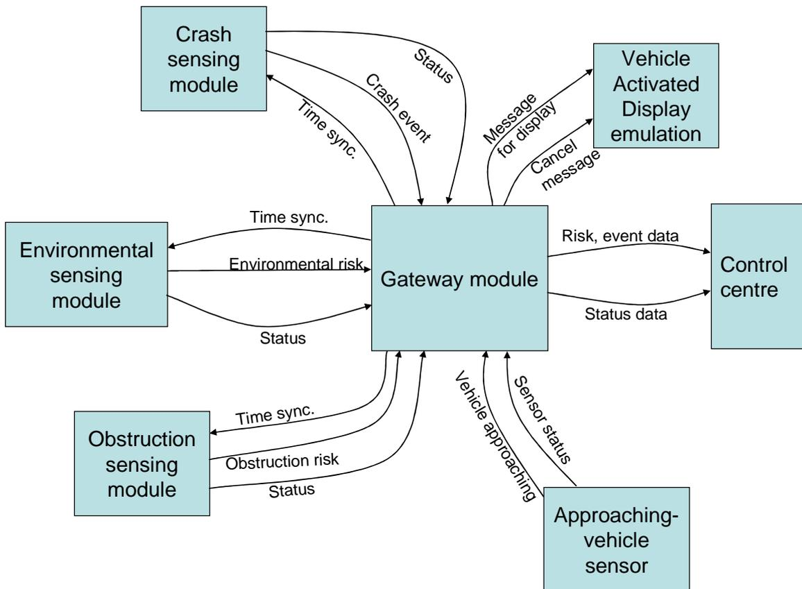
Figure 8: Gateway Message Traffic in Normal Operation
