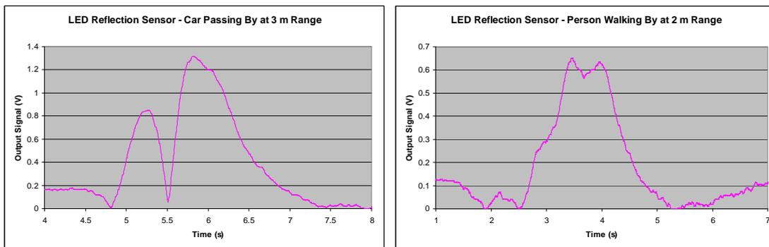
Figure 5 : Example Traces from Reflective Optical Stationary Obstruction Sensor
