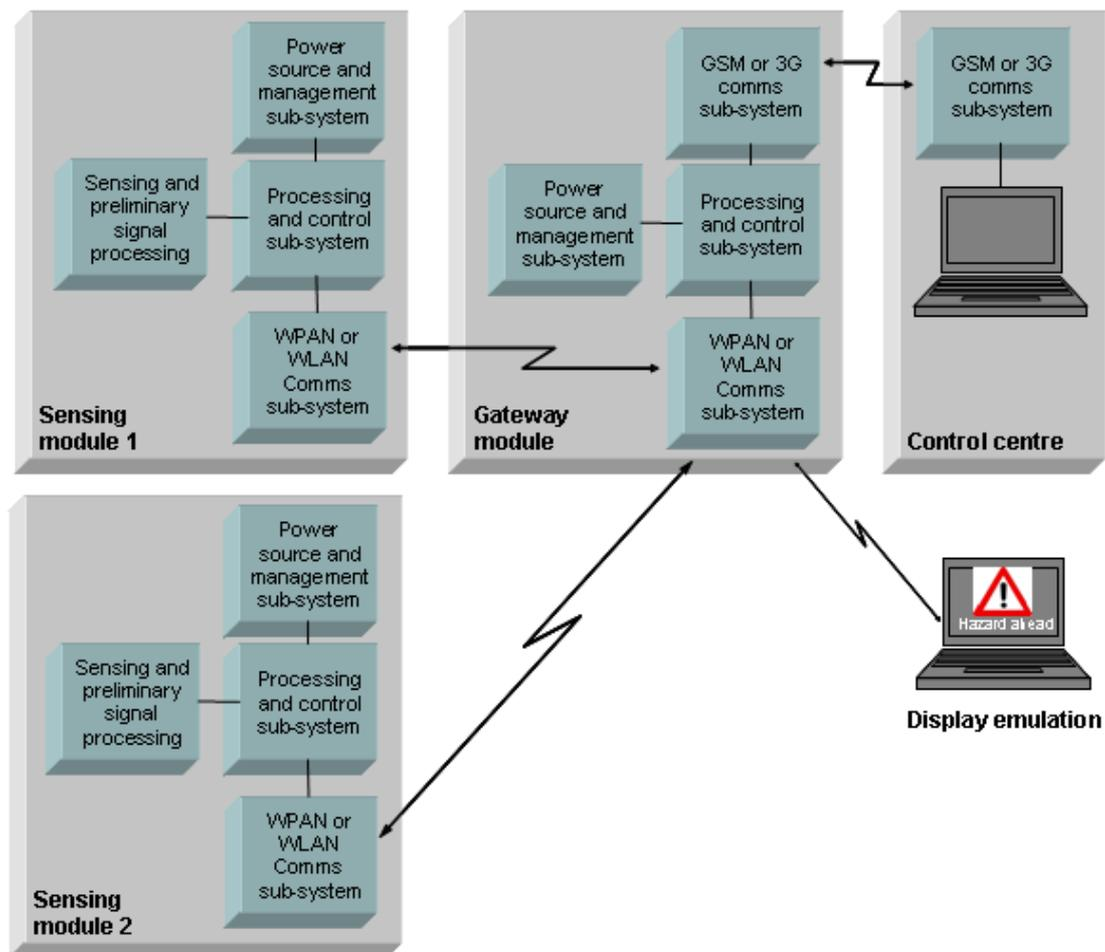
Figure 1: Top Level View of Smart RRS Primary Safety System
