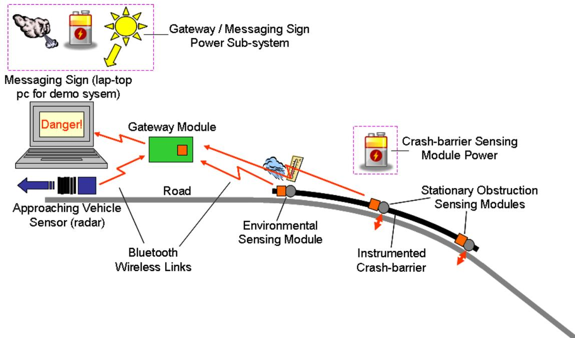
Figure 2 : Proposed Smart RRS Primary Safety System Configuration
