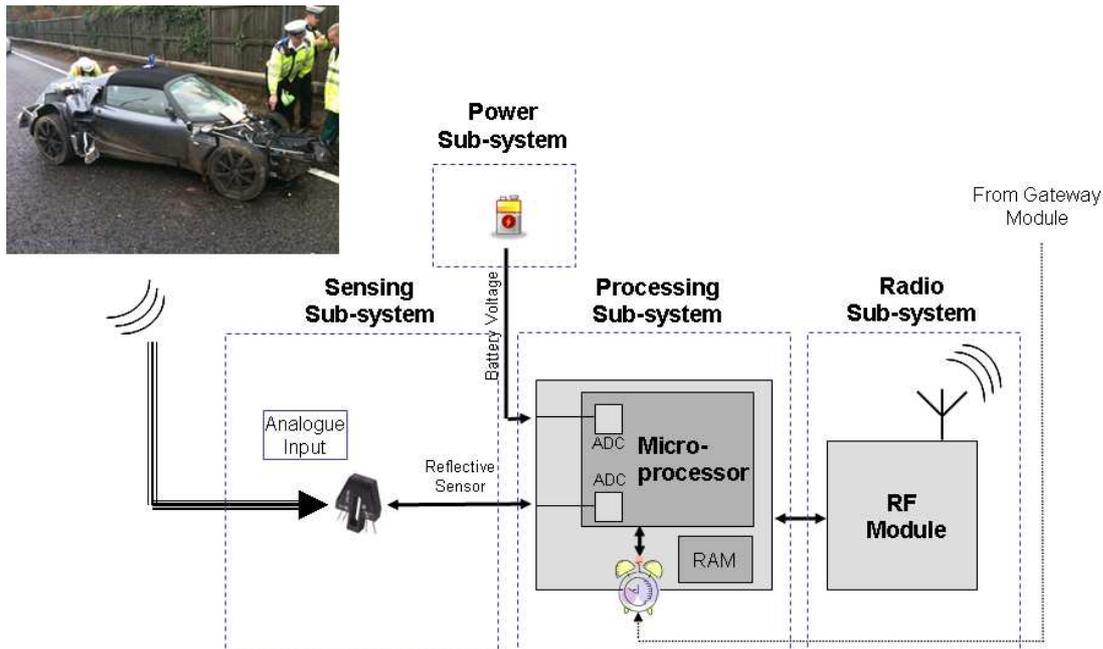
Figure 4 : Stationary Obstacle Sensing Module Configuration
