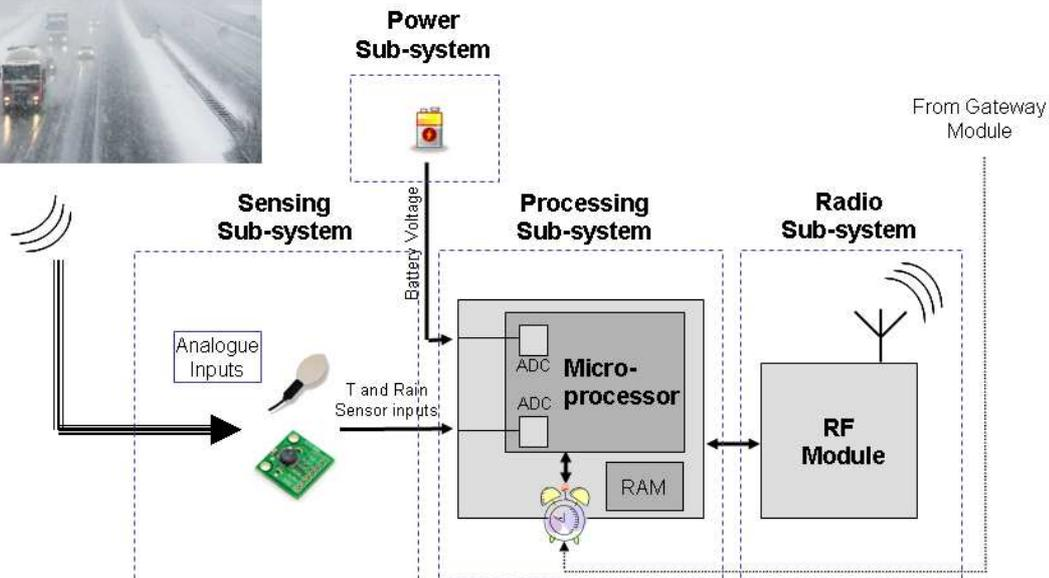
Figure 3 : Environmental Sensing Module Configuration
