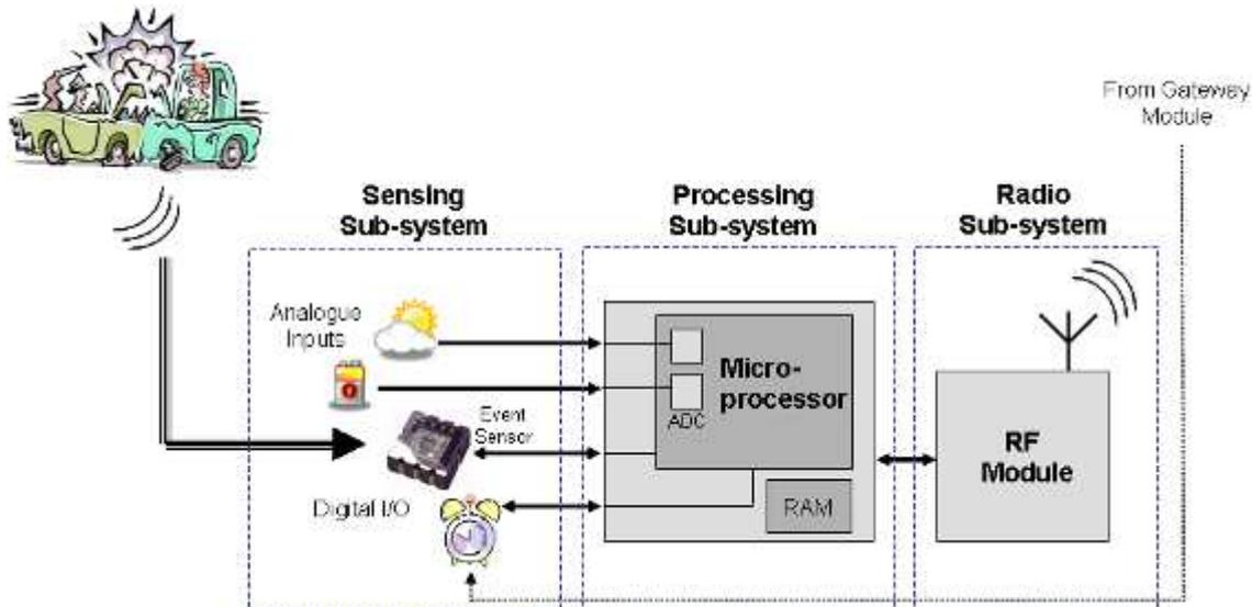
Figure 2 : Smart RRS Sensing Module Simplified Generic Architecture
