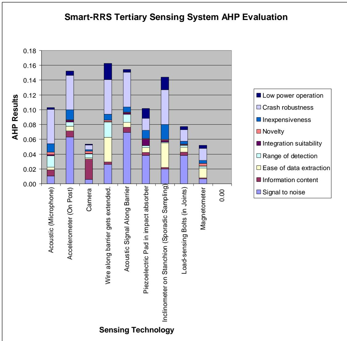
Figure 3: Results of AHP for Tertiary sensor selection<sup>3</sup>
