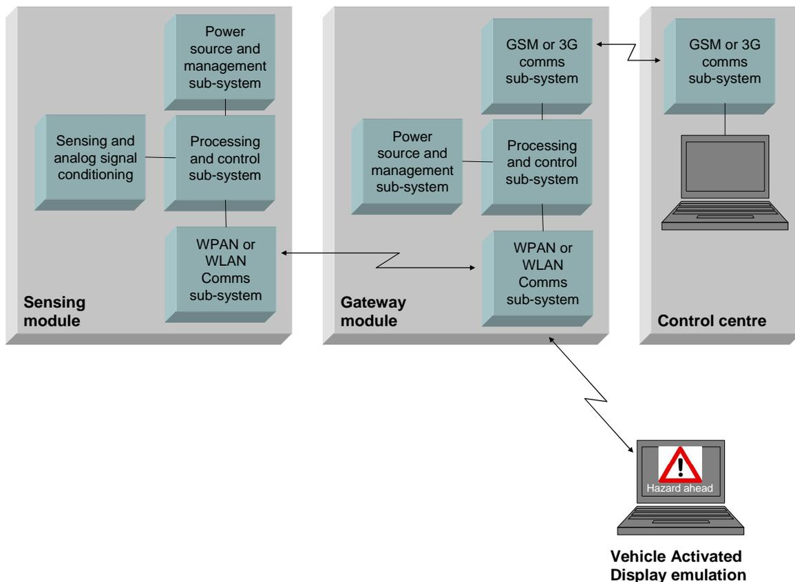
Figure 1: Top Level View of Tertiary Safety System
