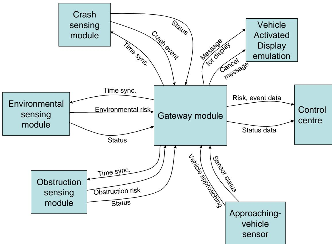
Figure 4: Gateway Message Traffic in Normal Operation
