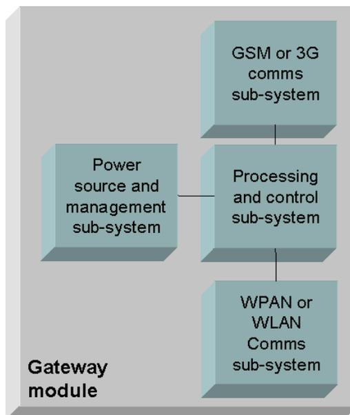
**Figure 5 : Gateway Module Generic Architecture**
