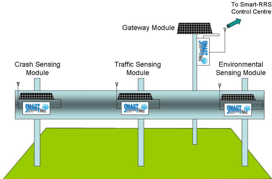
Figure 6 : Smart RRS Safety System Distribution
